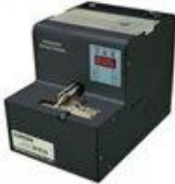
Introducing the new SFR30 Automatic Screw Feeder for automatic pick up of screws with a size range of M0.8~M3.0 screw head diameter 1.2~9.5mm with a length of 1.0mm~15mm. The digital display allows for easy and quick setting. The SFR30 Screw Feeder is able to deliver up to 50 pieces per minute.
